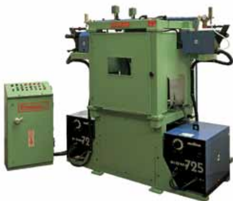
Saldatrice MIG coperchi compressori MIG welding machine for compressor covers
